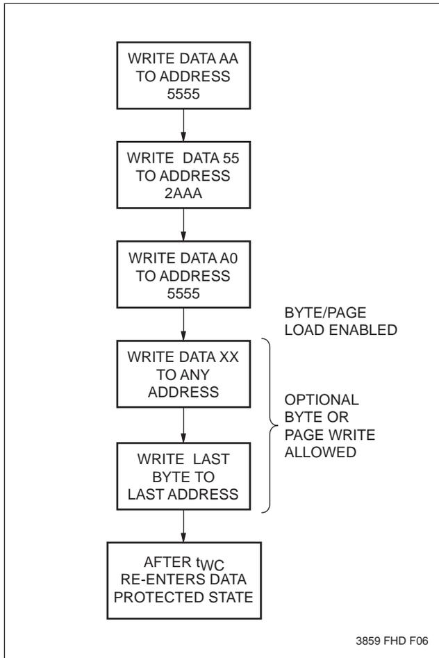
Regardless of whether the device has previously been protected or not, once the software data protection algorithm is used and data has been written, the X28HC256 will automatically disable further writes unless another command is issued to cancel it. If no further commands are issued the X28HC256 will be write protected during power-down and after any subsequent power-up.
