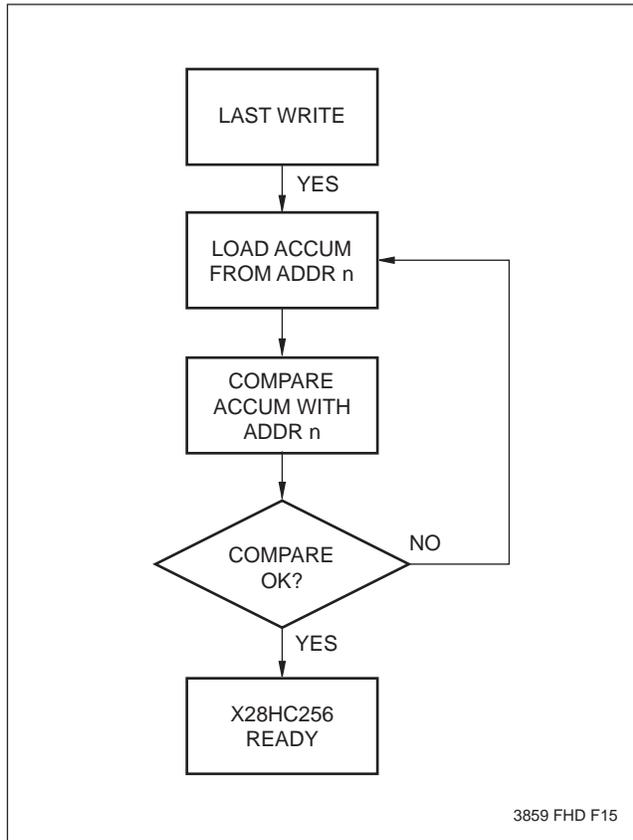
The Toggle Bit can eliminate the software housekeeping chore of saving and fetching the last address and data written to a device in order to implement DATA Polling. This can be especially helpful in an array comprised of multiple X28HC256 memories that is frequently updated. The timing diagram in Figure 4 illustrates the sequence of events on the bus. The software flow diagram in Figure 5 illustrates a method for polling the Toggle Bit.
