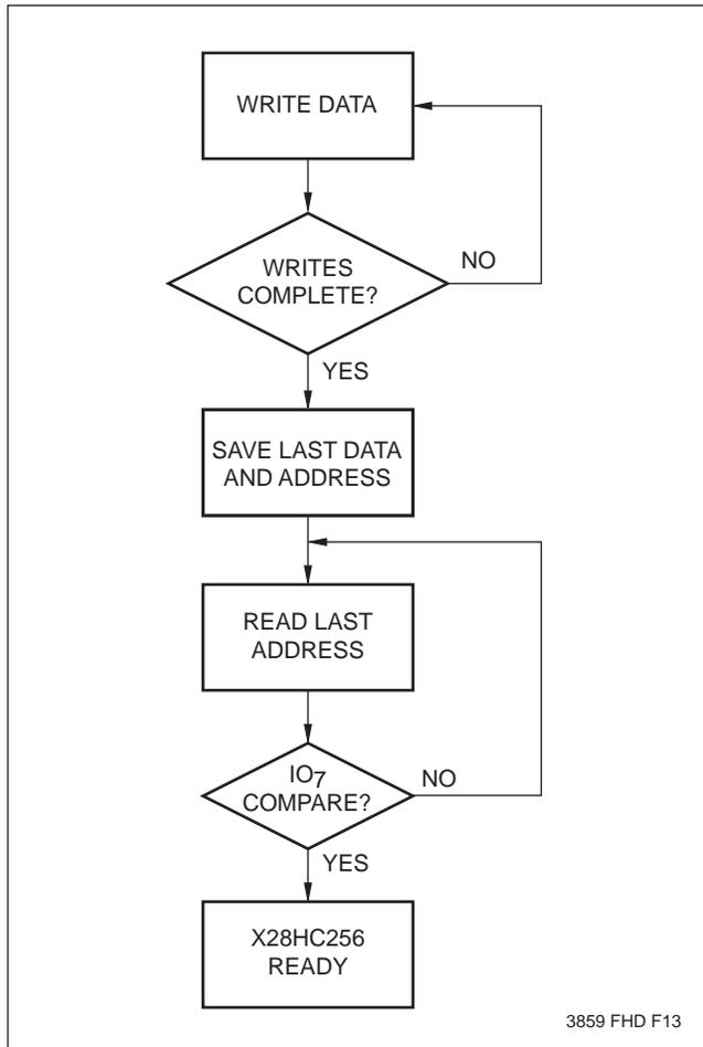
DATA Polling can effectively halve the time for writing to the X28HC256. The timing diagram in Figure 2 illustrates the sequence of events on the bus. The software flow diagram in Figure 3 illustrates one method of implementing the routine.
