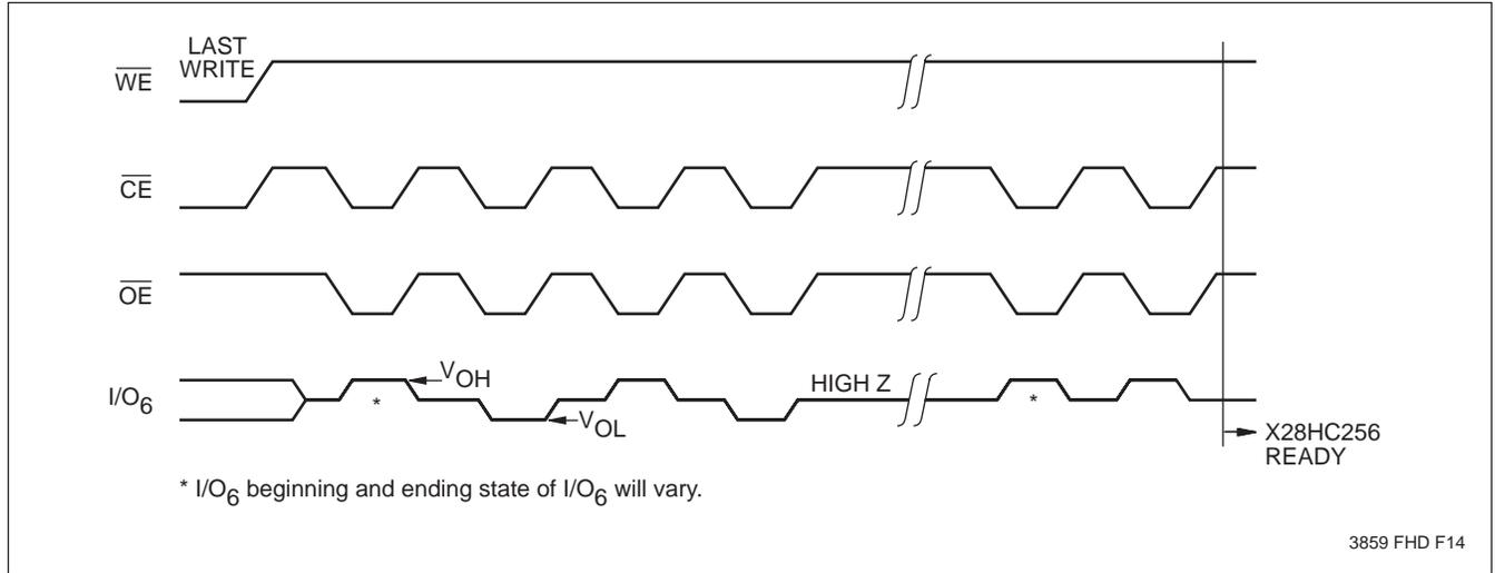
Figure 5. Toggle Bit Software Flow
