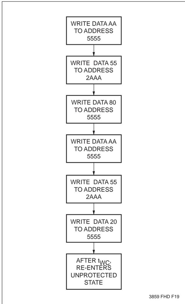
In the event the user wants to deactivate the software data protection feature for testing or reprogramming in an E2PROM programmer, the following six step algorithm will reset the internal protection circuit. After  $t_{WC}$ , the X28HC256 will be in standard operating mode.
