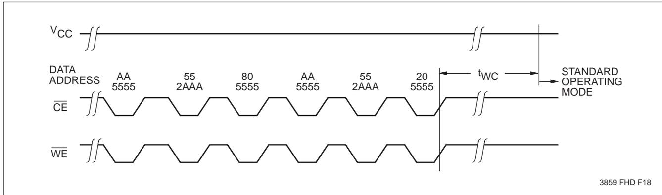
Figure 9. Write Sequence for resetting Software Data Protection
