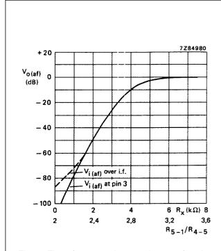
Fig.3 The a.f. output voltage at pin 8 as a function of the resistance values as shown in Fig.4.
