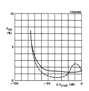
Fig.8 Total distortion as a function of the a.f. output voltage change. \_\_\_\_ 0 dB  $\cong$  900 mV over i.f. (pin 8)
