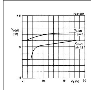
Fig.7 The a.f. output voltages at pins 8 and 1 as a function of the supply voltage; 0 dB  $\cong$  770 mV.
