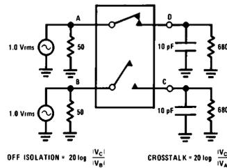
FIGURE 4. "OFF" Isolation, Crosstalk, Small Signal Response
