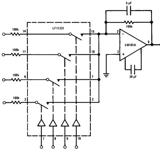
**8-Channel Analog Commutator with 6-Channel Select Logic**
