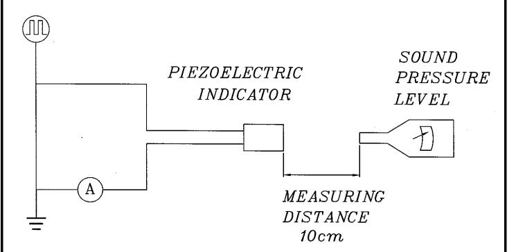
$\label{eq:mic_special} \mbox{Mic} \ : \mbox{RION S.P.L\,meter UC30 or equivalent}$
