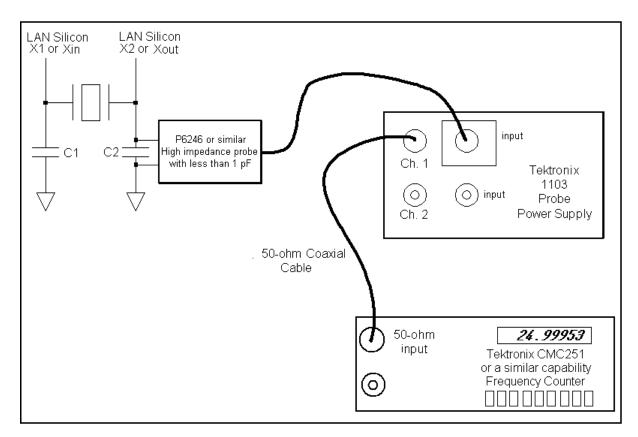
Figure 12. Direct Probing Method
