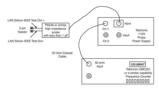
Figure 11. Indirect Probing Setup
