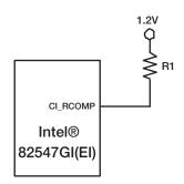
Figure 3. CSA port CI\_RCOMP Circuits
