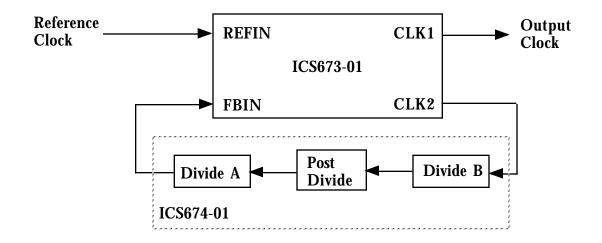
Note that in both examples Divide B is connected to the output of the ICS673. This is because Divide B has a higher operating frequency than Divide A.
