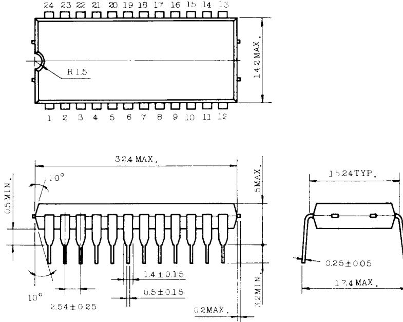
Note : Each lead pitch is 2.54mm. All leads are located within 0.25mm of their longitudinal position with respect to No.1 and No.24 leads.
