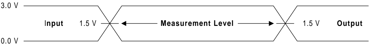
Figure 14. Input Waveforms and Measurement Levels
